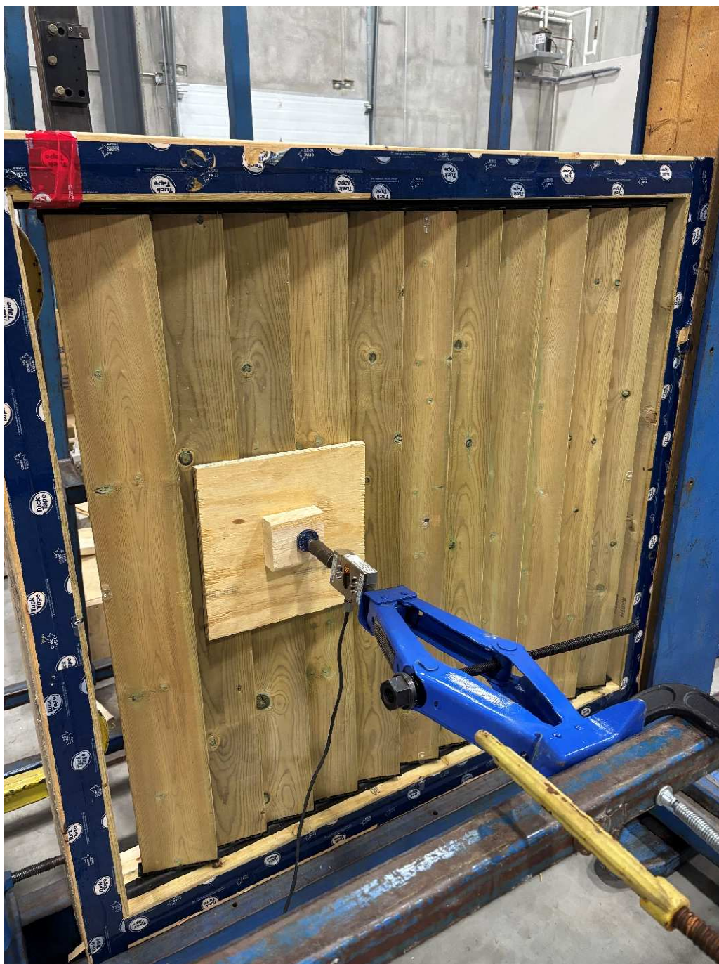
Figure A1: Flex-Fence® Sample with Static Load Applied
