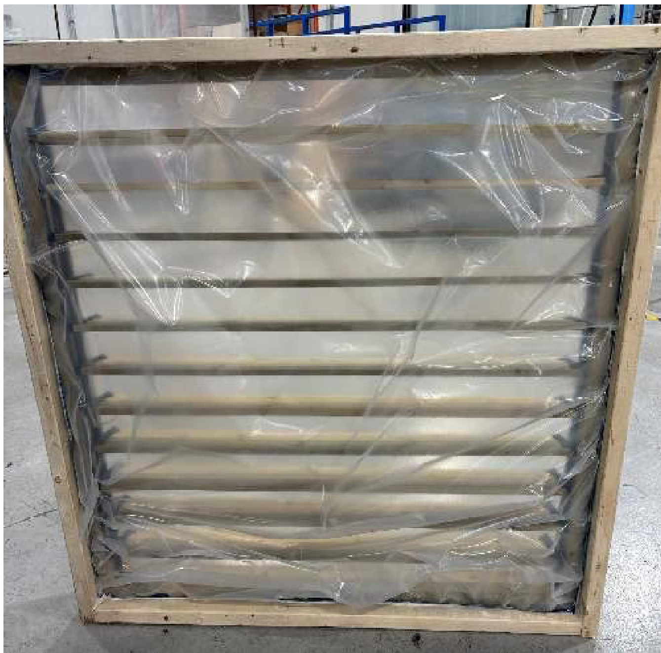
Figure A4: Structural Bag Installed on Back of Samples
