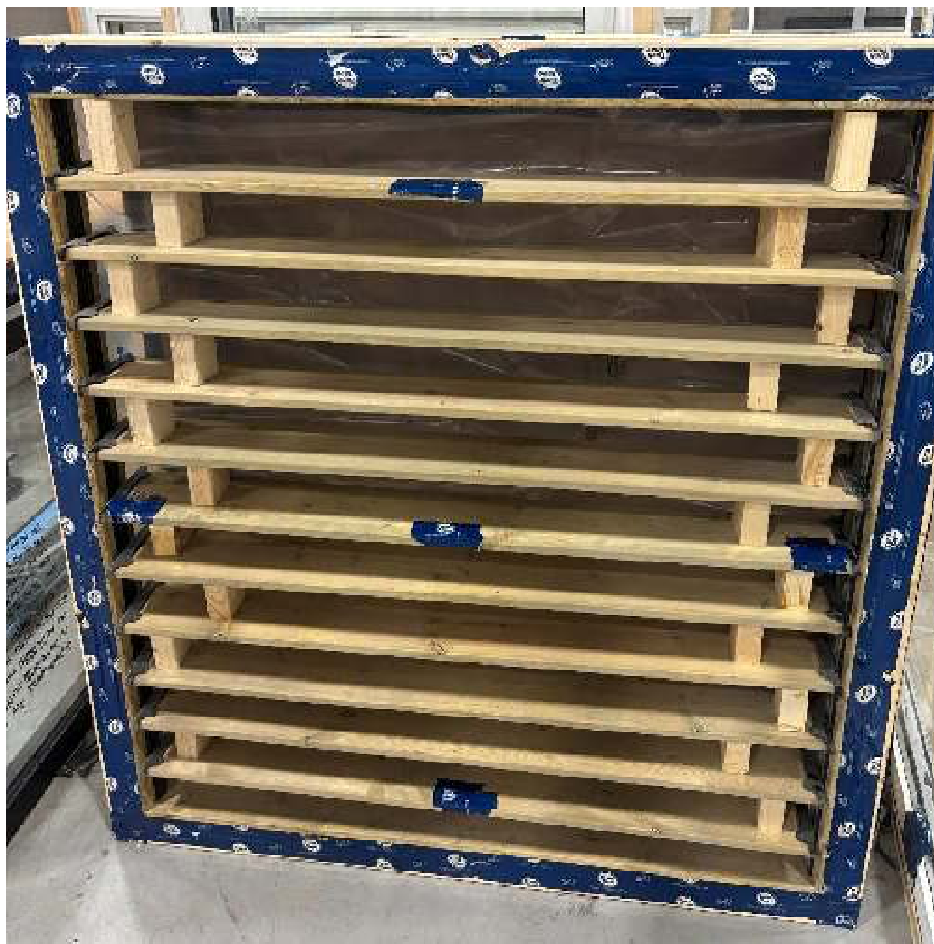
Figure A2: Flex-Fence® Sample 2, with Louvers Blocked Open
